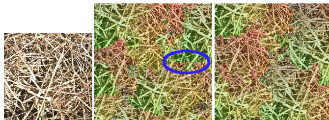
Fig. 3. Left: Sample texture. Middle: Synthesized texture without boundary avoidance. We have emphasized the patch boundaries by modulating each output pixel according to the position from which it was copied in the input image (thus, colour discontinuities correspond to patch boundaries). Notice the artifact in the middle right of the image where the input image boundary was hit on a line of successive pixels. Right: Synthesized texture with boundary avoidance.
