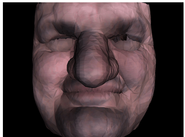
Figure 10. Extrusion (along surface normals) of surface from Figure 8 to create closed geometry.
