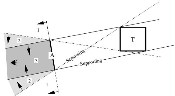
Figure 2: This figure shows occlusion in two dimensions (a planar cross section of 3D). Separating and supporting planes of an occluder  $A$  and an occludee  $T$  are shown, as is a synthetic viewpoint.
